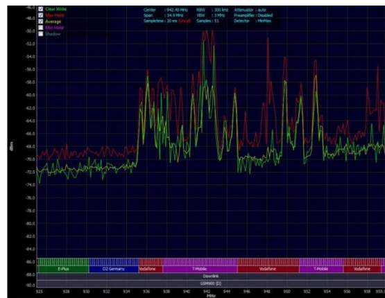
Figure 4: Frequency spectrum of GSM 900 taken in Lawipu
