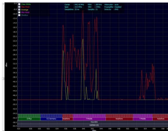
Figure 3: Frequency spectrum of GSM 900 taken in College veng
