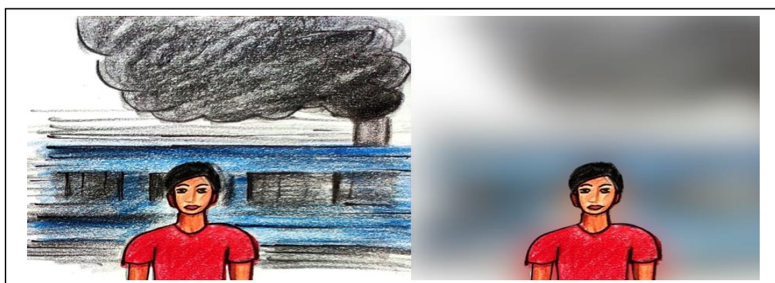
Figure 7: The conceptual diagram of moving grid where the first picture shows that a boy took a photo when the train behind him is at rest and the second picture shows that when the train is in motion thus blurring out the train in the picture. This is how moving grid works. Sketched by Miss Nandini Kashyap.
