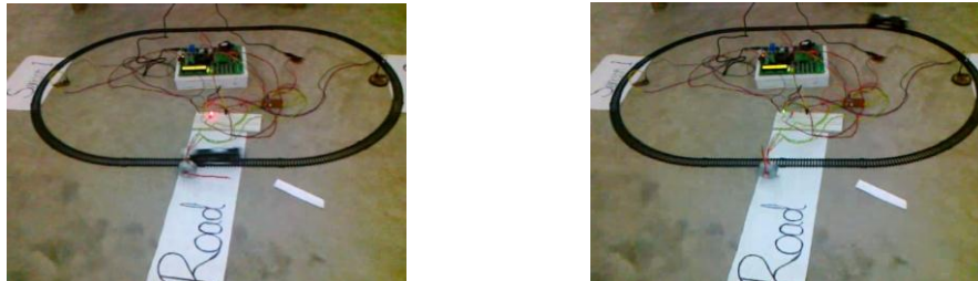
Figure 6: (a) shows when the train passes sensor 1, the gate is closed and (b) shows when the train passes sensor 2, the gate is opened.
