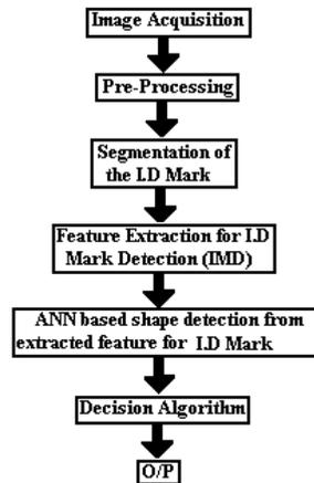
Figure 3: Flow diagram of proposed methodology.
