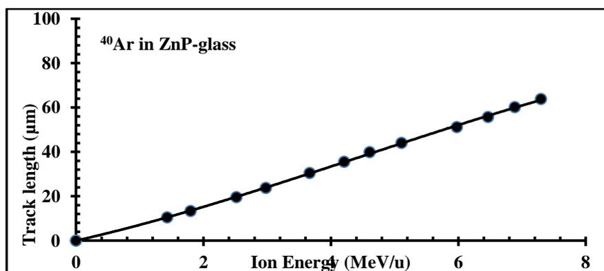
Figure 1: A Plot showing calibration curve between the energy of  $^{40}\text{Ar}$  and measured track length in ZnP-glass [7].
