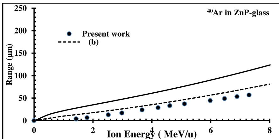
Figure 3: Measured range-energy data for  $^{40}\text{Ar}$  in ZnP-glass along with the theoretical values from (b) SRIM and (c) DEDXT program.
