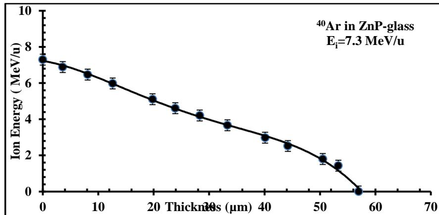
Figure 2: The energy loss curve for  $^{40}\text{Ar}$  in ZnP-Glass. The mean range of 7.3 MeV/u  $^{40}\text{Ar}$  in ZnP-glass is to  $57.0 \pm 2 \mu\text{m}$ .
