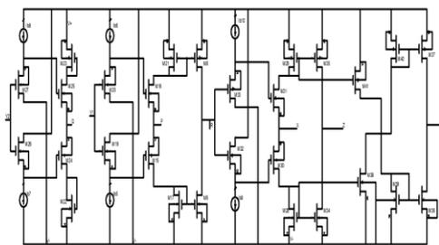
Fig 2: CMOS circuit of VG-DVDOCC
