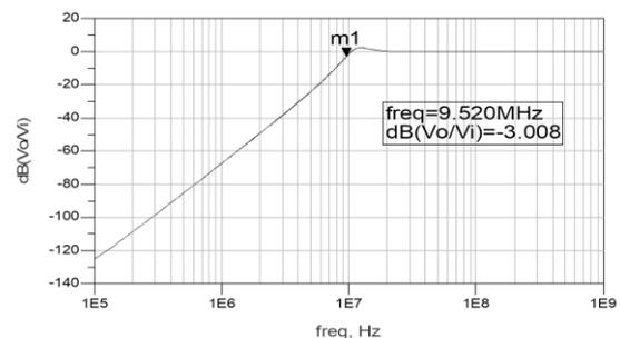
Fig 8: Frequency Response of high-pass filter
