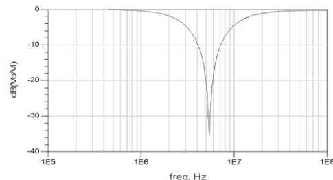
Fig 7: Frequency Response of Band-stop filter
