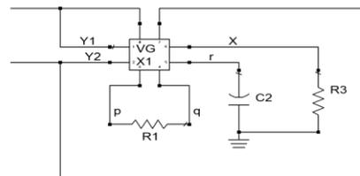
Fig 3: Floating Impedance converter based Active Inductor
