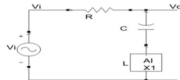
Fig 63: Band-stop filter
