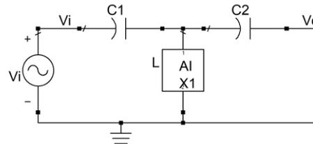
Fig 7: High-Pass Filter
