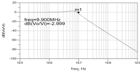
Fig 10: Frequency Response of low-pass filter
