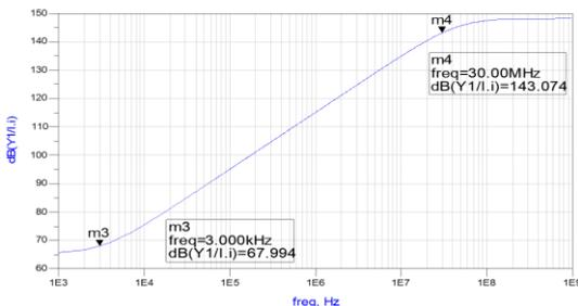
Fig 6: Frequency Response of Inductive Reactance of AI
