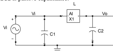
Fig 9: Low-pass Filter
