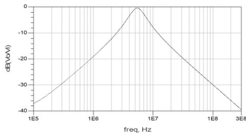
Fig 5: Frequency Response of Band-pass filter
