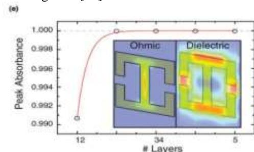
Figure 4 Ohmic versus dielectric loss in MPA [51].
