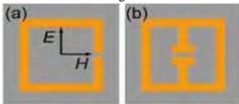
Figure 6: (a) Single split ring resonator (SRR) (b) Electronic split ring resonator (eSRR) [22].
