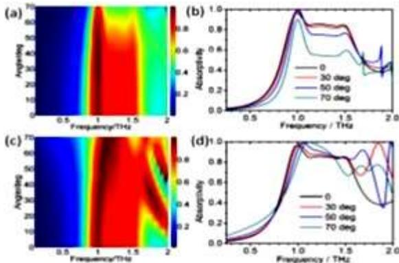
Figure 5: Simulated absorptivity for TE polarization. (b) and (d) for TM polarization. In (a) and (c) the x and y axes represent frequency and incident angle, respectively, and the absorptivity value is represented by different colors. (b) and (d) plot the absorptivity lines at selected incident angles of 0, 30, 50 and 70 degree[57].
