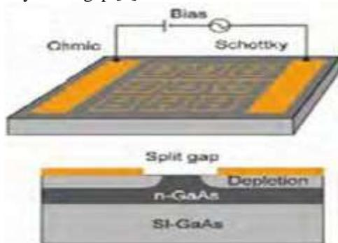
Figure 7: eSRR embedded in a conductive n-type GaAs substrate [7].
