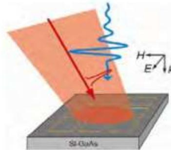
Figure 8. THz probe beam (blue) and femtosecond pump beam (red) incident on the Si-GaAs embedded metamaterial structure [7].
