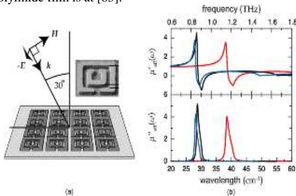
Figure10:Magnetically coupled SRRs (a) theTHz radiation incident on the SRRs at 30° from the normal. (b) The complex magnetic permeabilities of the structures simulated by using different geometries. [73]
