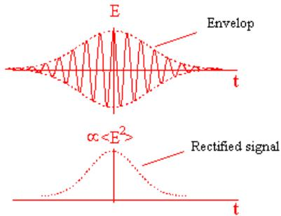
Figure 1. Optical rectification [21]
