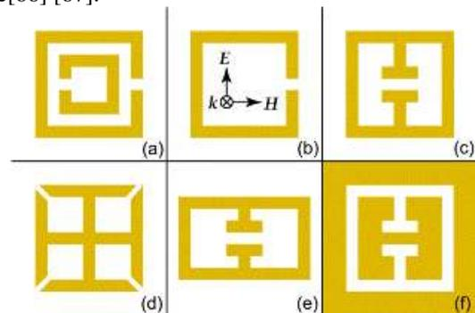
Figure 9. Some SRR variants at THz frequencies. (a) double SRR, (b) single SRR, (c) eSRR, (d) four-fold rotational-symmetry eSRR, (e) rectangular eSRR, and (f) complementary eSRR[63][64][65][66][67].
