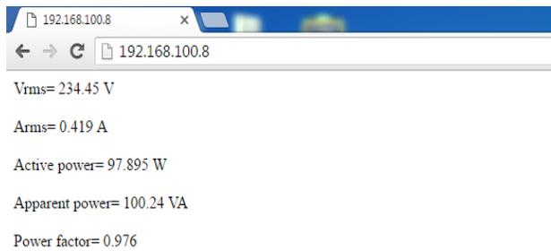
**Figure 14.** Viewing measured parameters through Wi-Fi on a web browser
