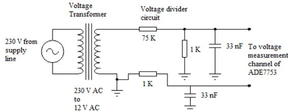
Figure 2. Connection to voltage channel
