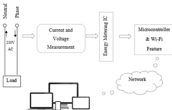
Figure 1. Block diagram of proposed meter
