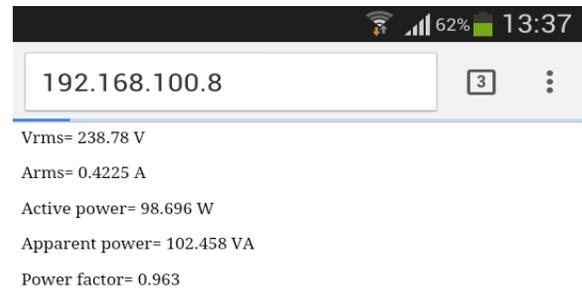
Figure 13. Viewing measured parameters through Wi-Fi on a mobile phone browser
