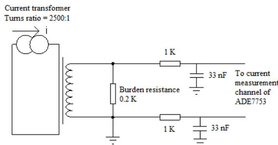
Figure 3. Connection to current channel
