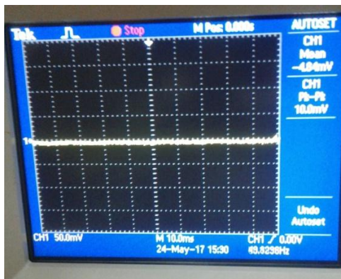
Figure: 6. Gate signal at MOSFET Q1 when battery is fully charged
