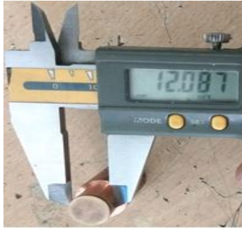
Figure1 (b) Size of electrode used (12 mm)
