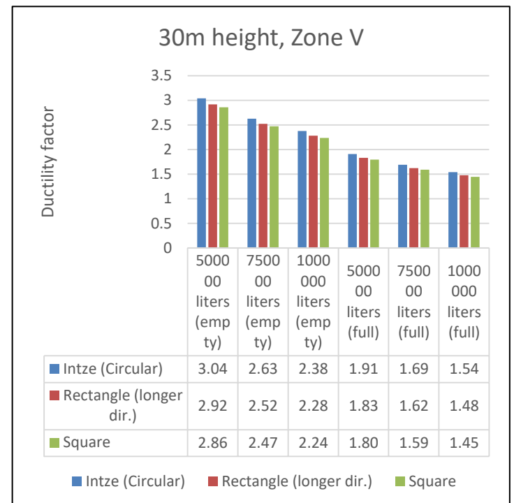
Figure 15: Ductility factor for 30m height, Zone V for different capacity and shape of container
