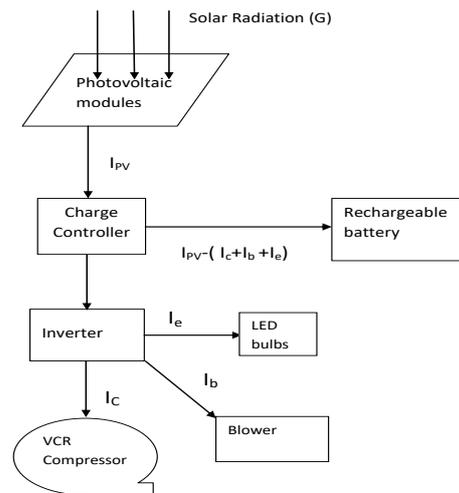
Fig.3. Schematic view of solar photovoltaic modules with charge controller, rechargeable battery and inverter for powering compressor, blower and LED bulbs during day time.
