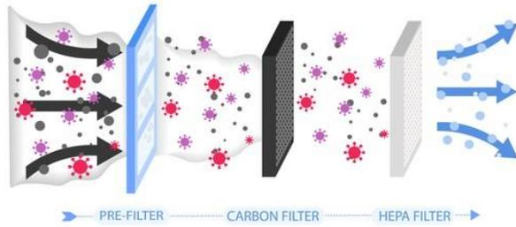
Fig.5. Schematic layout of air filter.[3']
