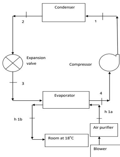
Fig. 2. VCR schematic with R134a as refrigerant for an office room to be maintained at 18°C for May
