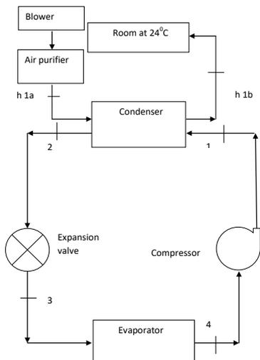
Fig. 1. VCR schematic with R134a as refrigerant for office room to be maintained at 24°C for January
