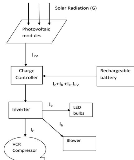
Fig.4. Schematic view of solar photovoltaic modules with charge controller, rechargeable battery and inverter for powering compressor, blower and LED bulbs during night time
