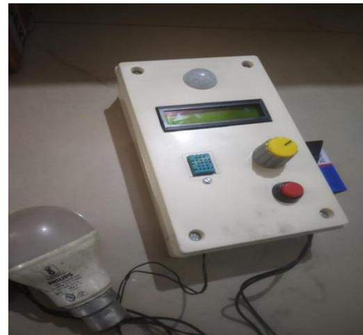
Fig 13: Final assembled Home Automation System
