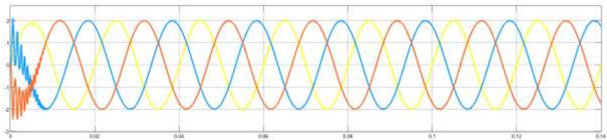
Fig. 6. Current under linear load
