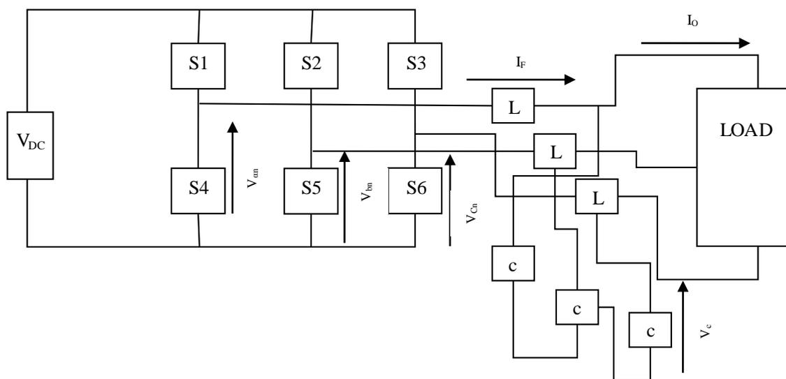
Fig. 1. Three Phase Inverter Control with LC filter for Renewable Energy Grid System
