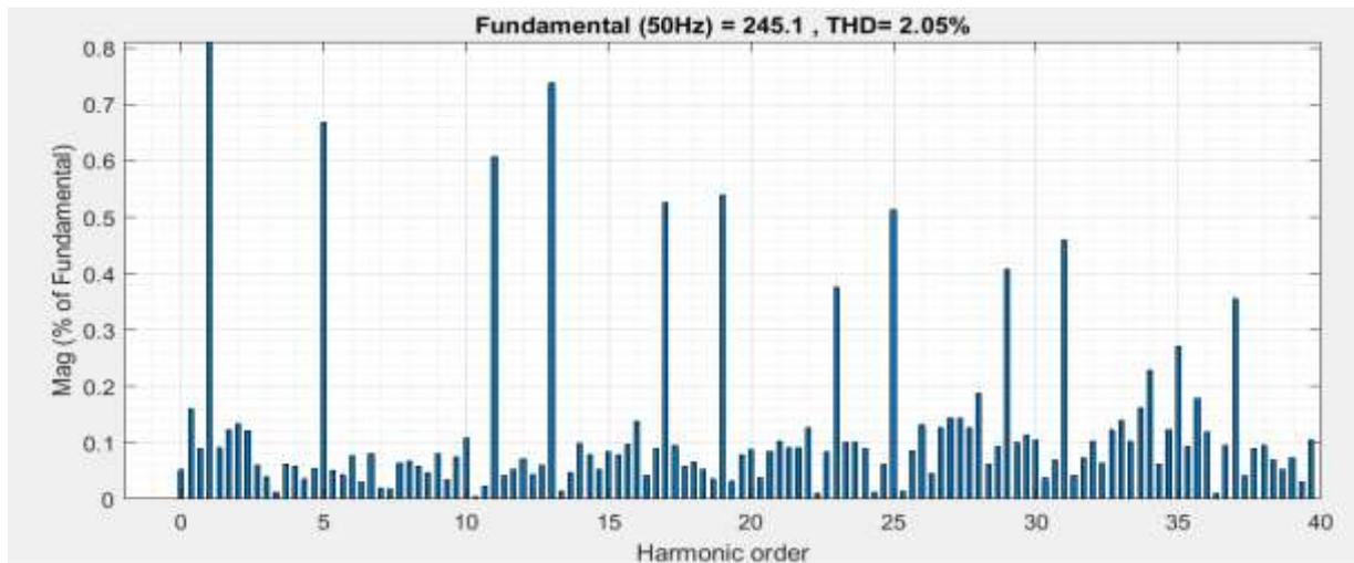
Fig. 8. Voltage THD under Non-Linear Load
