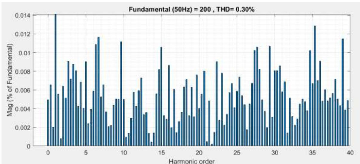
Fig. 5. Voltage THD under linear load
