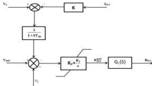
Fig.1. Model of svc controller
