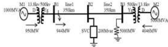
Fig. 5. Single line diagram of 2 machine 3 bus system
