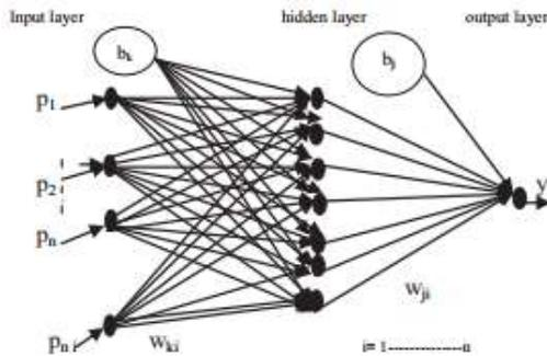
Fig.3. Architecture of multi-layer-feed forward ANN
