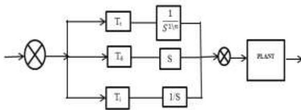
Fig .4. Block diagram of TID controller
