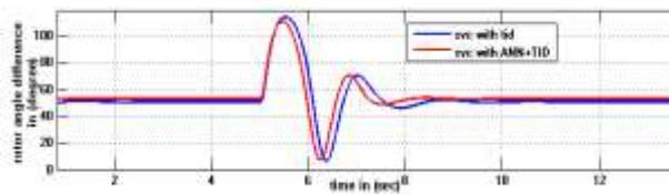
9. Rotor angle difference at generator
