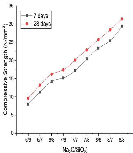
Figure 3 shown SiO<sub>2</sub> effect on compressive strength using line graph, in graph compressive strength at the curing period of 7 days and 28 days is shown. The percentage of GGBS keep constant at 30 % and also content of Na<sub>2</sub>O keep constant (6 %, 7 %, 8%) to form different combination with the variation of SiO<sub>2</sub> (6 %, 7 %, 8%) content, as shown in figure on X-axis. . Compressive strength varies from 8.00
