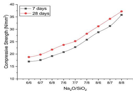
Figure 4 shown SiO<sub>2</sub> effect on compressive strength using line graph, in graph compressive strength is represented at the curing period of 7 days and 28 days. The percentage of GGBS keep constant at 40 % and also content of Na<sub>2</sub>O keep constant (6 %, 7 %, 8%) to form different combination with the variation of SiO<sub>2</sub> (6 %, 7 %, 8%) content, as shown in figure on X-axis. . Compressive
