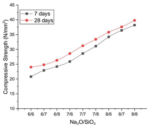
Figure 5 shown SiO<sub>2</sub> effect on compressive strength using line graph, in graph compressive strength at the curing period of 7 days and 28 days is shown. The percentage of
