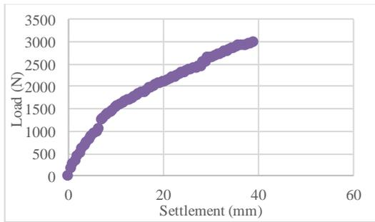
Figure 6: Load settlement curve stone column 225mm length
