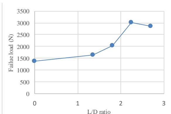
Figure 9: Failure load at different L/D ratio
