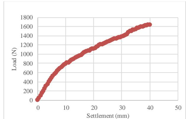
Figure 4: Load settlement curve stone column 135mm length
