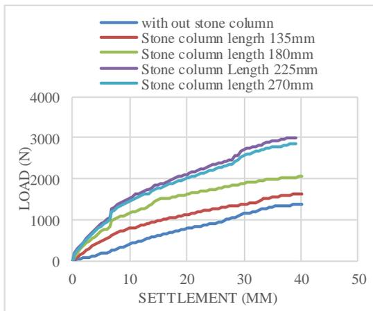
Figure 8: Load settlement curve comparison for different length of stone column
