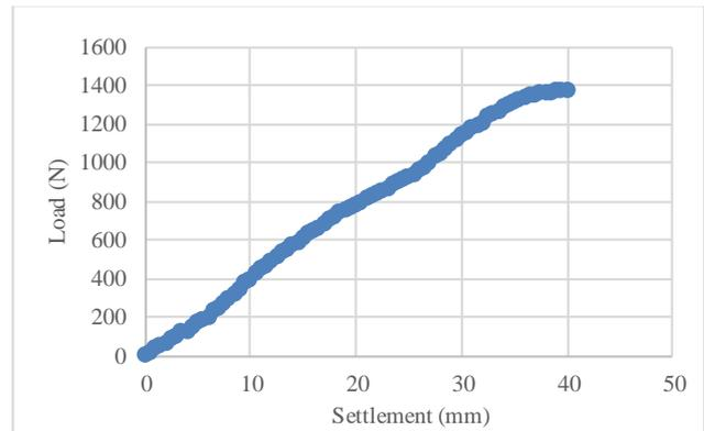
Figure 3: Load settlement curve without stone column
