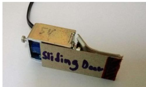
Fig. 25. Door is opened by solenoid pulling in action for enrolled user
