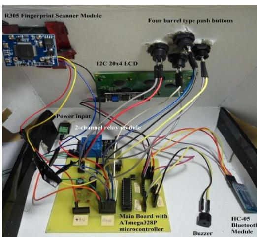
Fig. 22. Internal structure of the demonstration box
