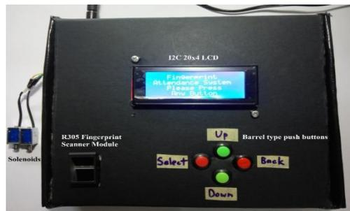
Fig. 23. Exterior of the demonstration box
