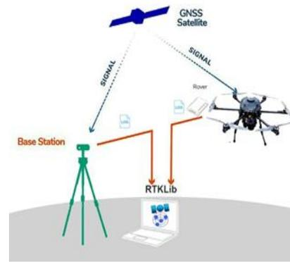
Fig. 2. PPK method for data processing.
