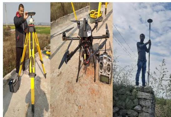
Fig. 6. Base setup for GNSS receiver, UAV, and GCP marking.
