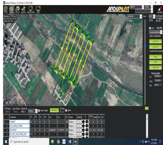
Fig. 5. Flight plan in mission planner for the area of interest.
