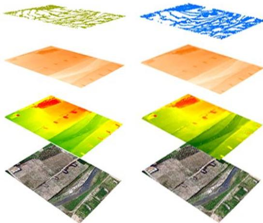
Fig. 9. Geospatial data models are generated by Pix4D by processing (left) RTK data (right) PPK data.
