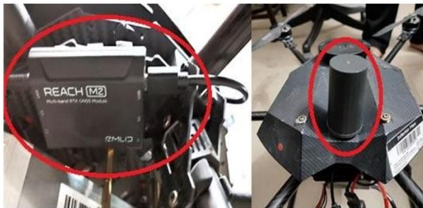
Fig. 4. Reach M2 multi-band GNSS receiver with SMA antenna.
