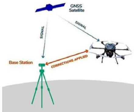
Fig. 1. RTK method for applying the correction.
