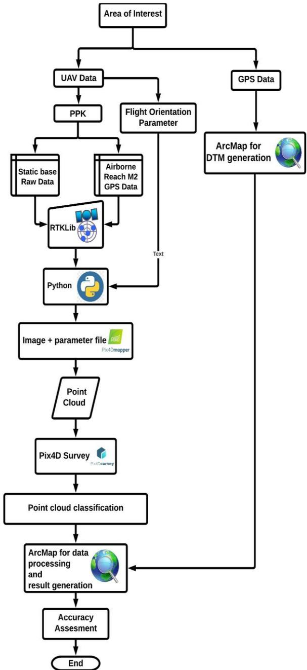
Fig. 8. Flow diagram of a methodology for accuracy assessment.
