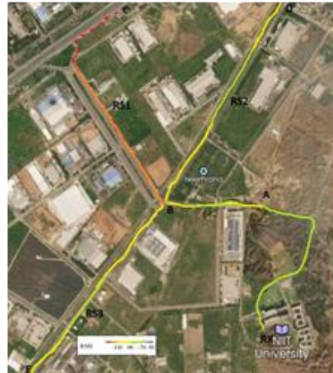
Fig. 3. The RSSI level heat map for different segment of road with distance.
