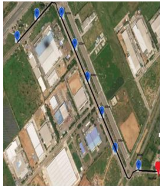
Fig. 8. Mobility scenario experimental setup where road segment divided into small segment of 100 m
