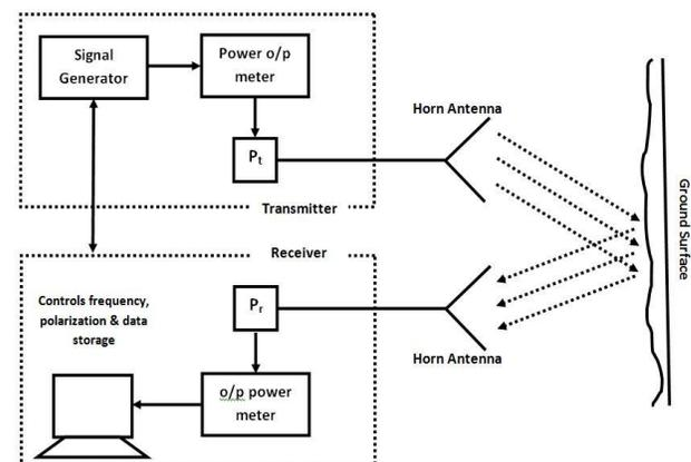
Figure2: Block diagram of active microwave sensor.
