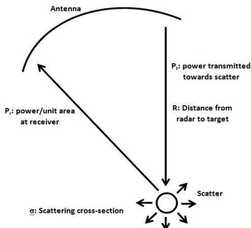
Figure1: Concept of radar equation.
