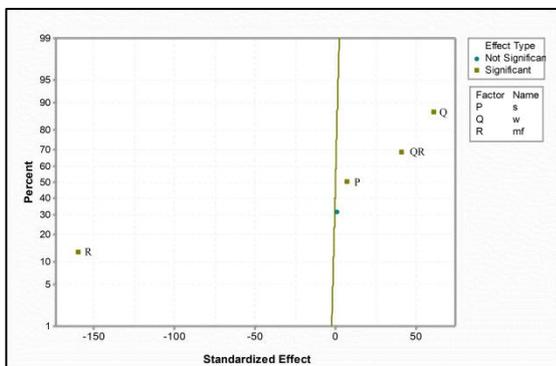
Fig. 5(b). Normal probability plots of effects for  $\eta_{mech}$
