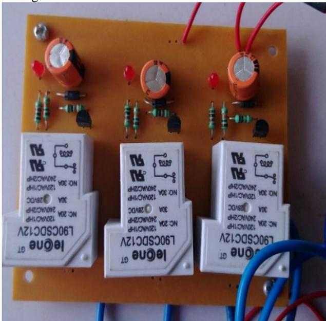
Fig.2. Relays interfaced to PV module for Isc and Voc measurement
