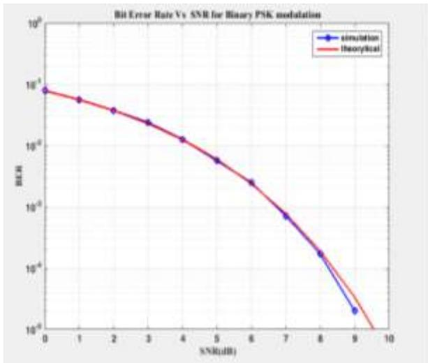
Fig.5 Bit error rate Vs SNR for BPSK modulation
