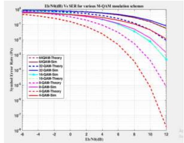
Fig. 7 Symbol error rates for M-QAM modulation schemes
