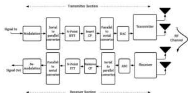
Fig. 2 Basic MIMO-OFDM system
