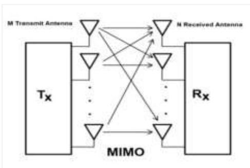
Fig.1 Multi Input Multi Output antenna system
