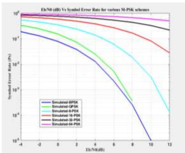
Fig. 6 Symbol error rates for M-PSK modulation schemes
