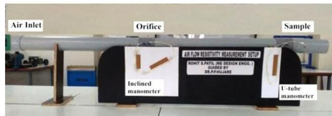
Figure 6. Experimental Setup for Flow Resistivity Measurement
