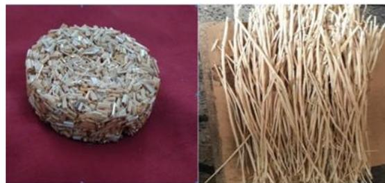
Figure 4. Test Sample and raw material of wheat straws
