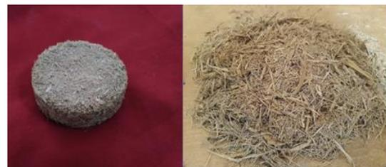
Figure 3. Test Sample and raw material of sugarcane fibers
