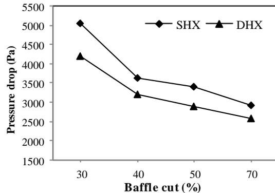
Fig. 8. Variation of pressure drop with baffle cut.
