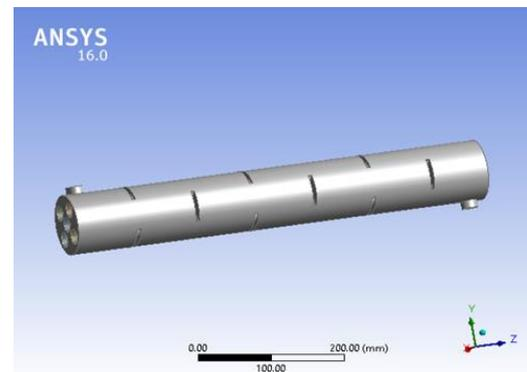
Fig. 2. Double segmental baffle heat exchanger.
