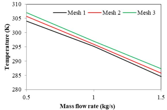
Fig. 3. Mesh Independence for temperature
