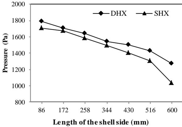
Fig. 4. Pressure along the length of shell side of heat exchanger.
