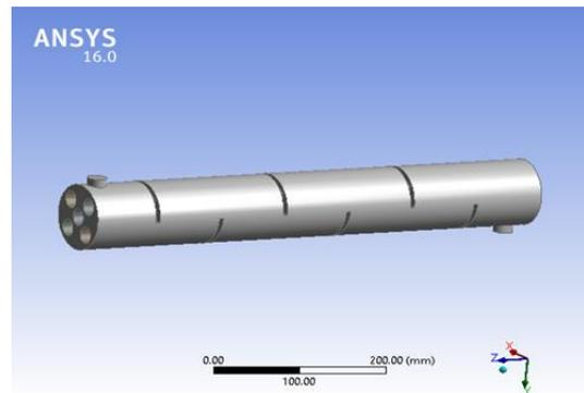
Fig. 1. Single segmental baffle heat exchanger.
