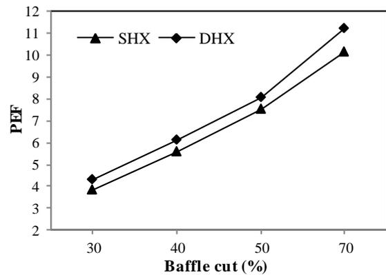
Fig. 10: Variation of performance evaluation factor with baffle cut.
