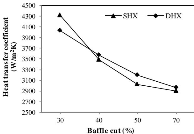
Fig. 9. Variation of heat transfer coefficient with baffle cut.
