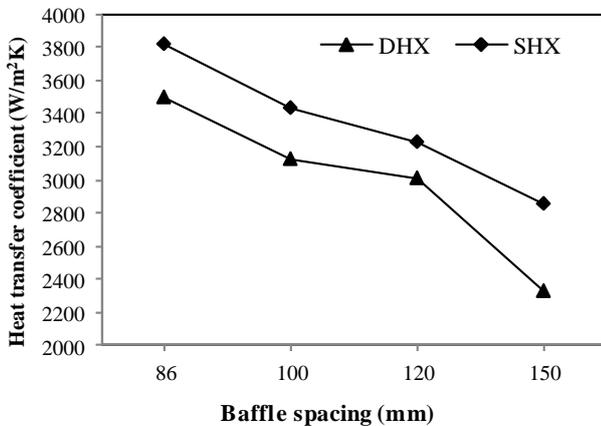
Fig. 6. Heat transfer coefficient with baffle spacing.
