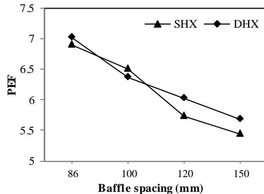
Fig. 7. Variation of PEF with baffle spacing
