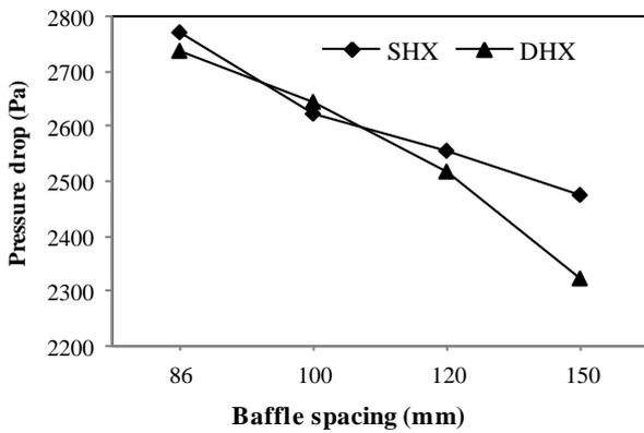
Fig. 5. Variation of pressure drop with baffle spacing.
