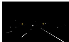
Fig. 7: Grayscale Image with Extracted Lane Lines
