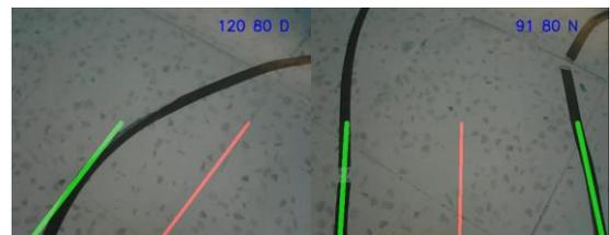
Fig. 23: Lanes Detected by Hardware
