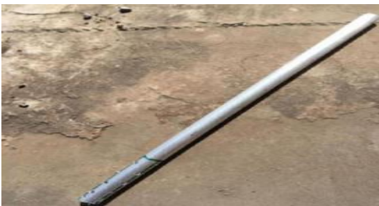
Fig. 5. Perforated aluminum pipe for gas collection
