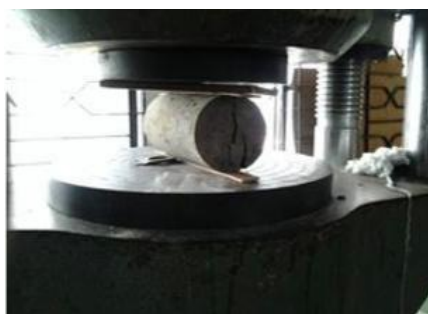
Fig. 6. Split Tensile strength test
