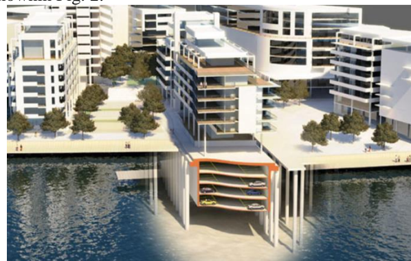
Fig. 2. A model section showing how the prefabricated concrete caissons provide large submerged parking areas in four levels [17]
