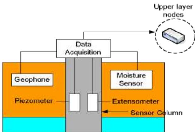
**Figure4:** WSN deployment with sensor column [32]
