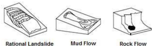
**Figure1:** Illustration of some of the major types of landslide movement [3]
