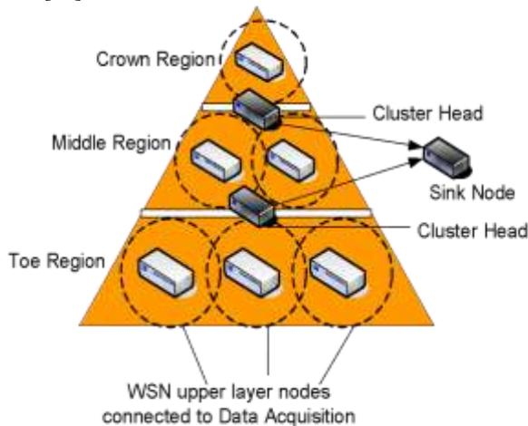
**Figure5:** Regionalized WSN architecture for landslides [32]
