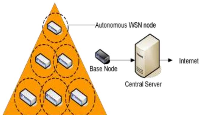
**Figure6:** Autonomous WNS architecture for landslides [35]
