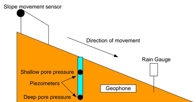
Figure3: Placement of landslide monitoring sensors [31]
