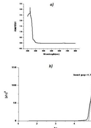
Figure 3: a) Absorption spectra b) tauc plot of ZnO nano particle using conventional method.
