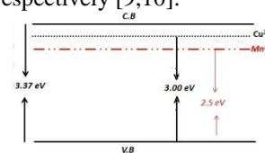
**Figure 2:** Band structure after doping ZnO with manganese and cooper
