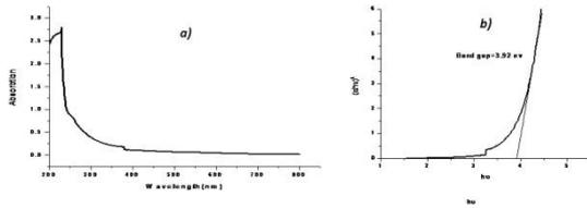
**Figure 4:** a) Absorption spectra b) tauc plot of ZnO nano particle using fast crystallization method.
