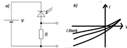
**Figure 1:** a) Schematic circuit diagram of a photodetector.
