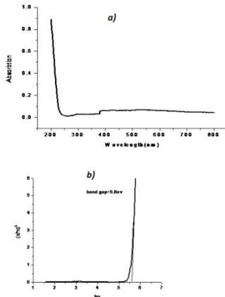
**Figure 5:** a) Absorption spectra and b) tauc plot of ZnO nano rod.
