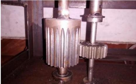
Figure 2: Gears mounted of different face widths
