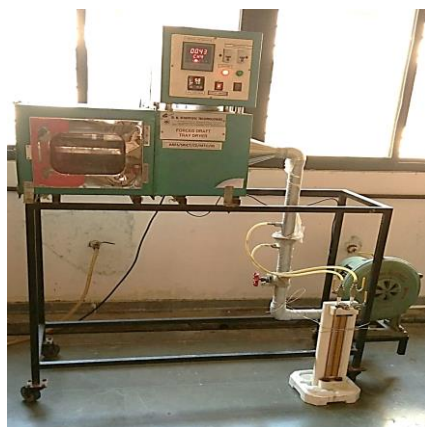
Fig. 2. Working of convective tray dryer
