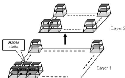
**Figure 6:** HCM Network structure Source: Ref[6]
