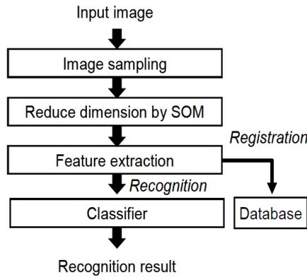
**Figure 2:**General procedure of face recognition algorithm using Self-Organizing Map (SOM) Source:Ref[2]
