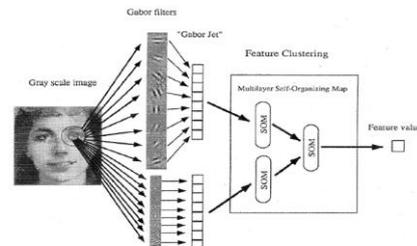
**Figure 3 :**Feature extraction and compression, Source:Ref[3]
