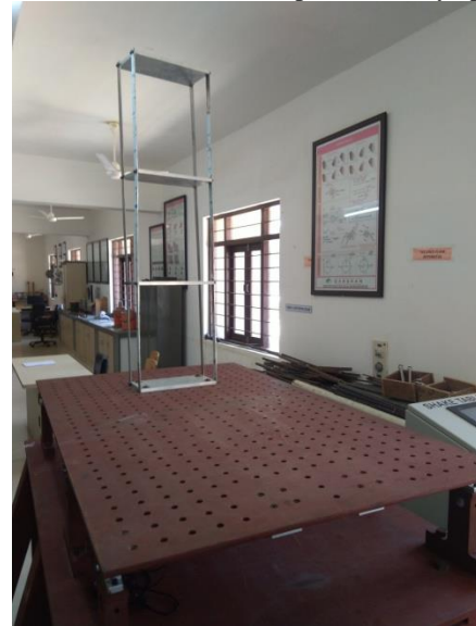
Fig. 2. Experimental setup – Seismic shaking table and model under test.
