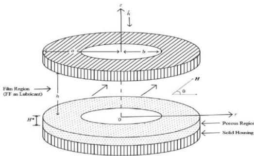
Fig.1. Porous annular discs squeeze film
