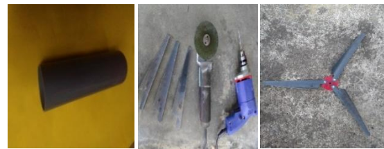
Fig. 2: Construction Stages of Wind Turbine Blades
