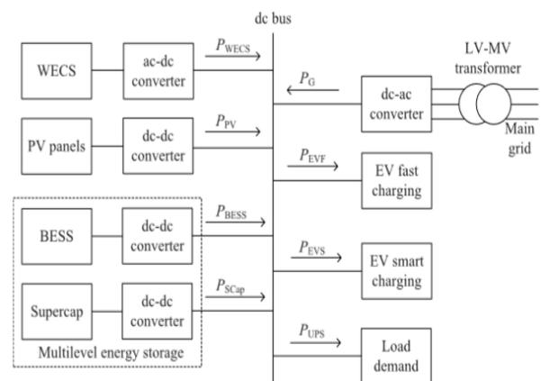
Fig. 1: Layout of a DC microgrid [1]
