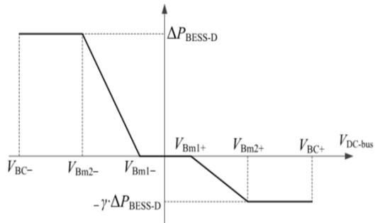
**Fig. 5:** Droop control of the BESS to mitigate the power deviations of DC microgrid in higher than the scheduled SOC of the BESS [1]
