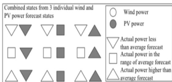
**Fig. 4:** Aggregation of wind and solar power forecast in microgrid [1]
