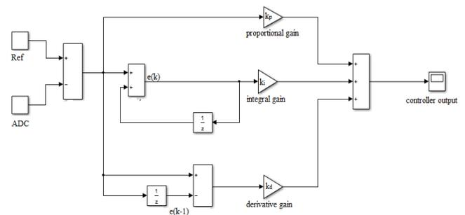
Figure 6: Block diagram of digital PID controller.
