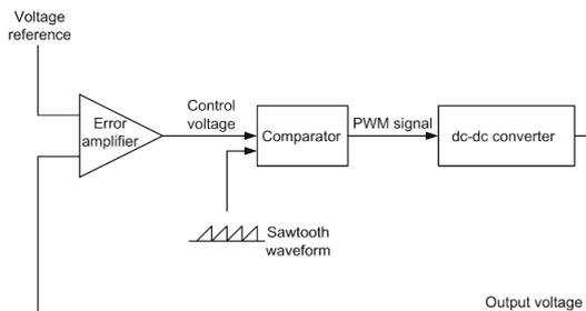
**Figure 4:** Control schemes for dc-dc converters: Voltage-Mode Control [13]
