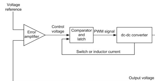
**Figure 5:** Control schemes for dc-dc converters: Current-mode Control [13]
