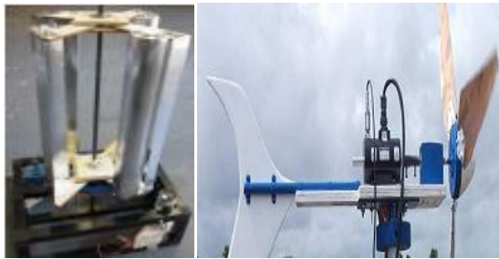
Fig. 1: Vertical and Horizontal Axis Wind Turbine [1, 5].
