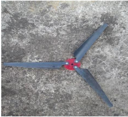
Fig. 4: Horizontal Axis Micro wind turbine blade under study
