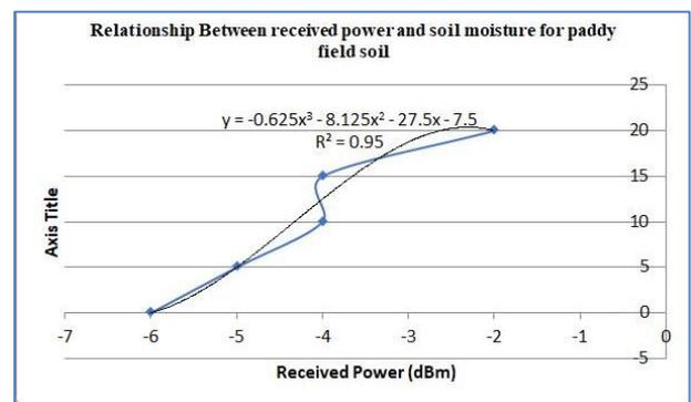
**Fig. 12:** Relationship Between received power and soil moisture for Paddy field soil
