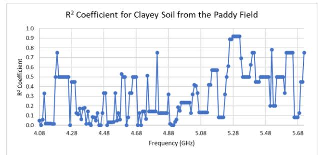
**Fig. 11:** Relation between frequency and R<sup>2</sup> Coefficient for clayey Soil from the Paddy Field
