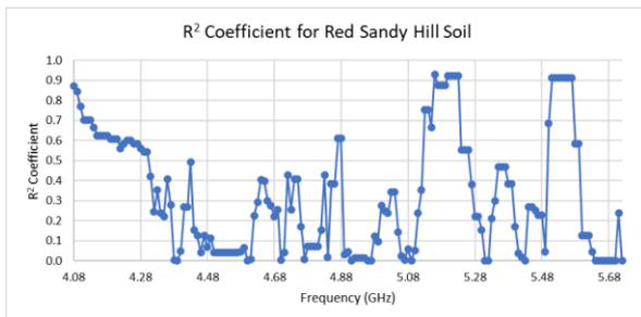
**Fig. 9:** Relation between frequency and R<sup>2</sup> Coefficient for Red Sandy Hill Soil
