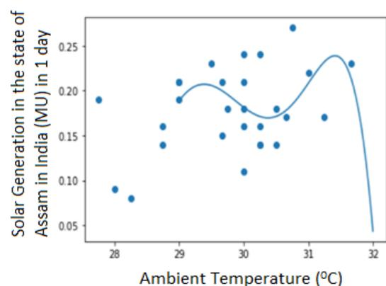
**Figure 2:** Polynomial regression plot solar generation (net MU) versus ambient temperature [4]
