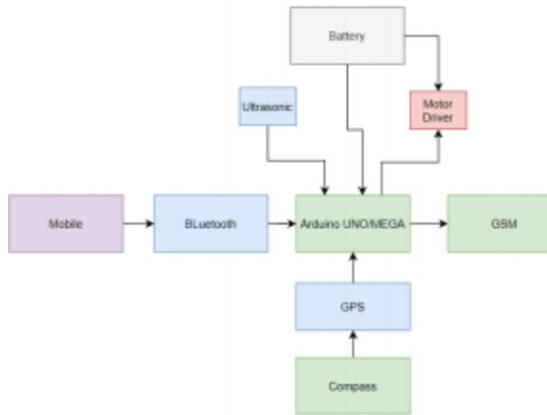
Fig. 5: Block Diagram
