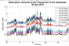
**Figure 5:** Total Attenuation of different frequency channels of Radiomter
