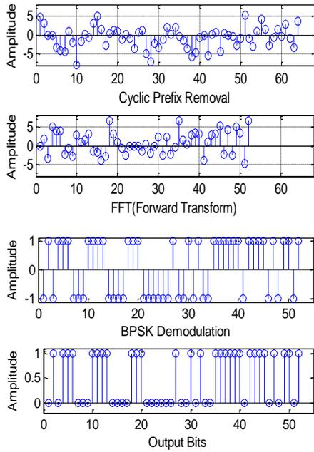
Figure 9: OFDM Receiver Processing Blocks
