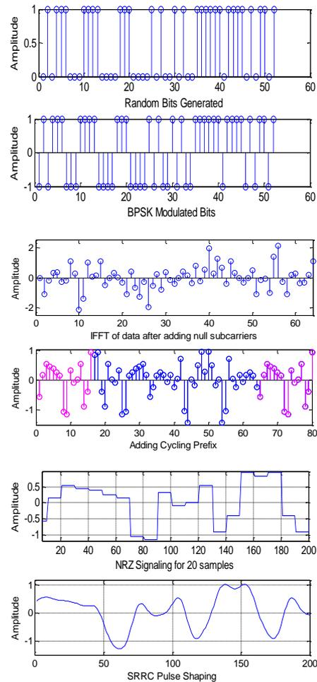
**Figure 7: OFDM Transmitter Processing Blocks**
