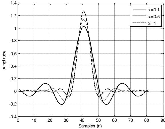
Figure 4: Impulse response for SRRC filter [18].
