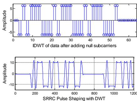
**Figure 13:** SRRC Filter used with DWT-OFDM
