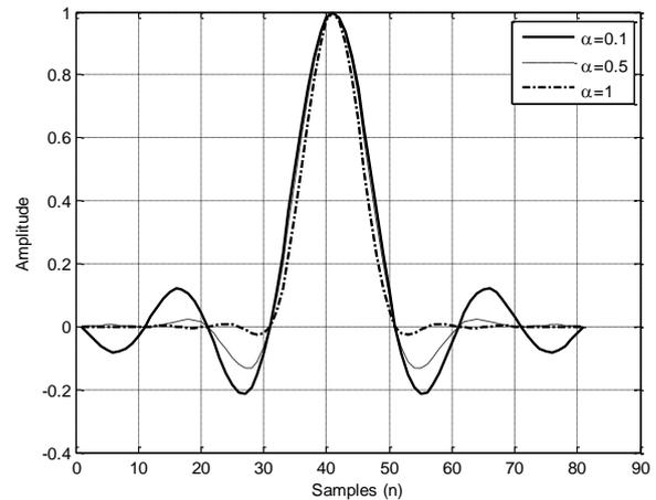
Figure 3: Impulse response for RC filter [16].
