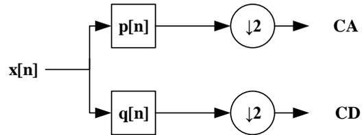
Figure 1: Filter-analysis of a one dimensional DWT [24]
